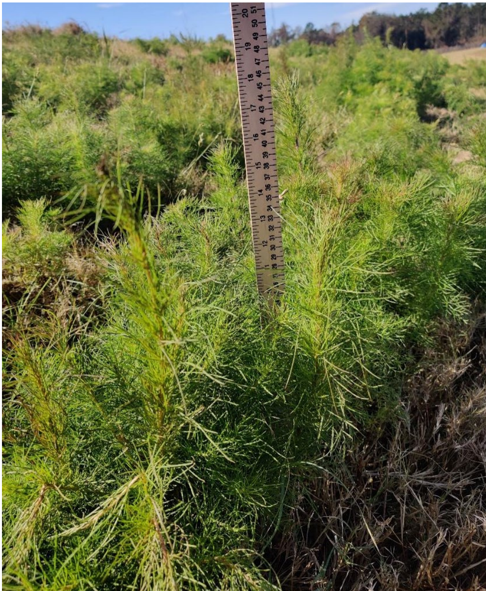
Figure 8. Weed Height Greater than 6 inches Observed on Northern Slope of the CCR Landfill
