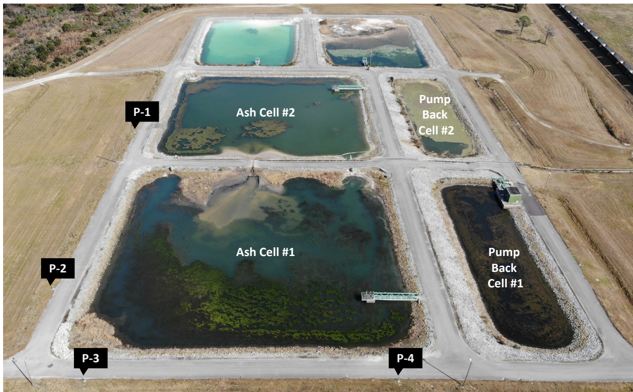
Figure 1. Layout of the CCR Surface Impoundment System, Adjacent Pump Back Cells, and Piezometers
